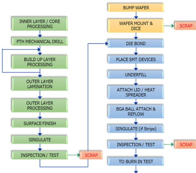
Figure 1. Flip Chip Process
