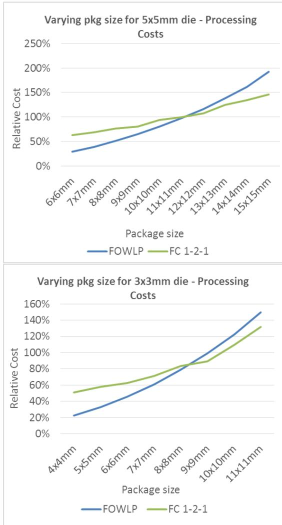
Figure 3. Varying Package Size
