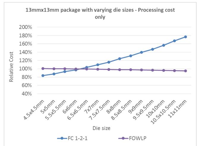
Figure 4. Varying Die Size – Processing Cost Only
