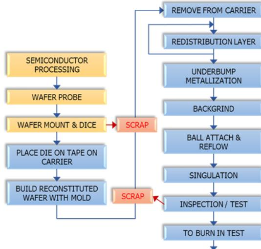
Figure 2. Fan-out Wafer Level Packaging Process
