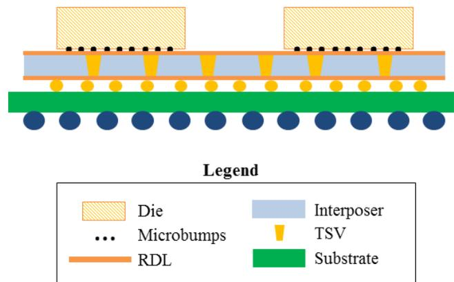
**Figure 2.** 2.5D Cross-section
