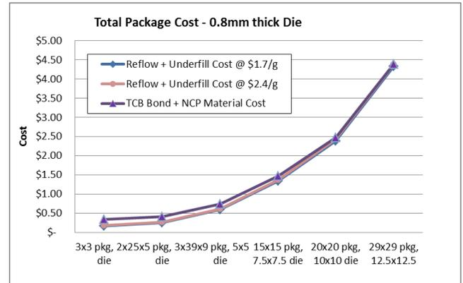
Figure 1 – Total Package Cost for 0.8mm Thick Die
