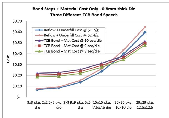
Figure 6 – Cost of Bond Steps at Different TCB Speeds
