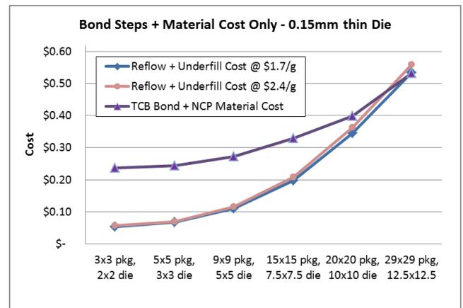
Figure 3 – Cost of Bond Steps Only for 0.15mm Thin Die
