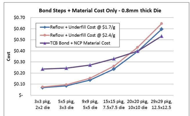
Figure 2 – Cost of Bond Steps Only for 0.8mm Thick Die
