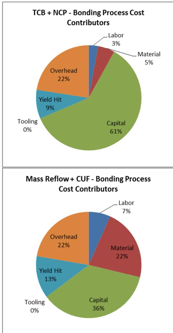
Figure 4 – Bonding Process Cost Contributors
