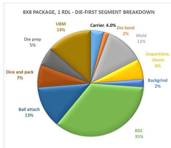
Figure 1 – Die-first Segment Breakdown
